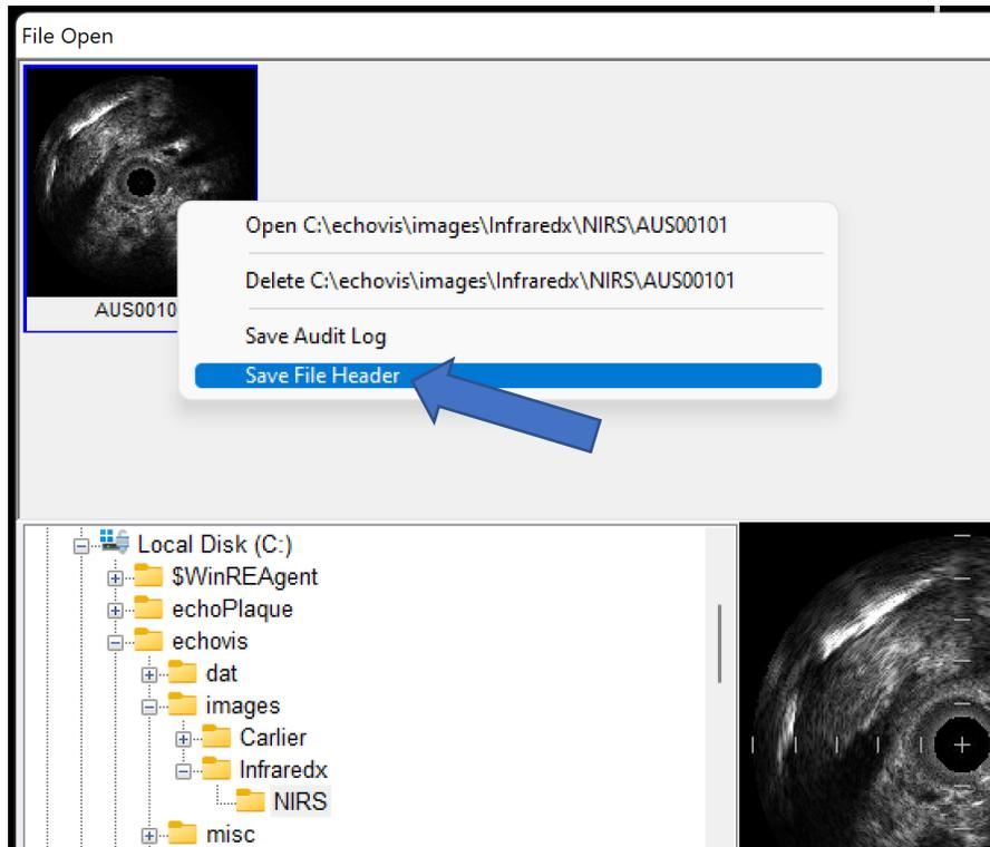
Left click on “Save File Header” to save the header. By default, a text version of the header will be saved in the same folder as the DICOM pullback you have selected.
